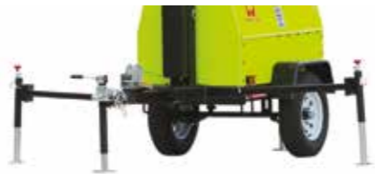
Four stabilizers with manual rotation for travel configuration
