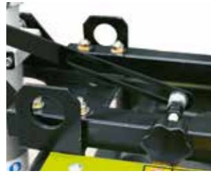
Mast support and four rings for lifting
