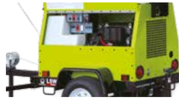
Manual control panel and integrated fuel tank
